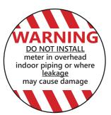
**Caution:** These water meters are not recommended for installation in uninsulated suspended ceilings where freezing is possible, or in any overhead indoor piping configuration where leakage may cause damage.
