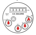
The **3/4" meter** has a fourth dial, as shown above. The x0.01 dial is used for 20 P/G and 10 P/G rates.Note: The 3/4" meter has a 5 digit totalizer.
