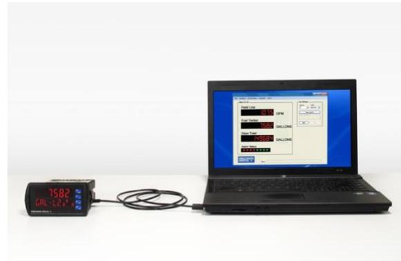
*The controller can be powered from the USB connection. When using the USB connection, **DO NOT** apply AC or DC power to the controller.*
