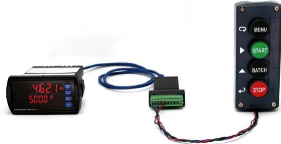
Figure 22. Controller to Control Station Connection
