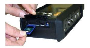
Simply remove the card, insert into your PC and copy the log files over. The files are conveniently formatted in Excel and Microsoft Text Doc formats.
