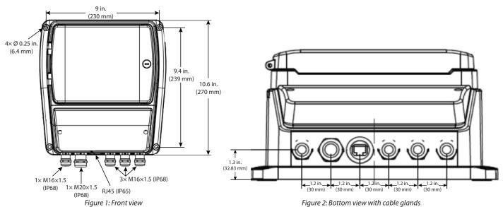
Figure 2: Bottom view with cable glands
