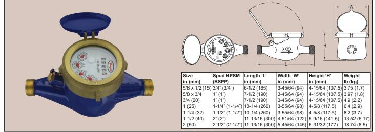
**The Series WM2 Multi-Jet Water Meter** is ideal for commercial and industrial applications. The multi-jet design allows for simplicity and accuracy with wide flow ranges, even in low flow applications. The magnetically driven, hermetically sealed register will not leak or fog and is completely separated from the water. These water meters are designed for long service life and maintenance-free operation, even under harsh conditions.
